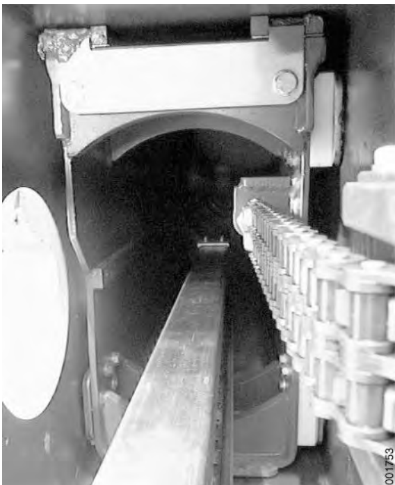
The diagram shows inner slide plates in the attachment's main beam.
