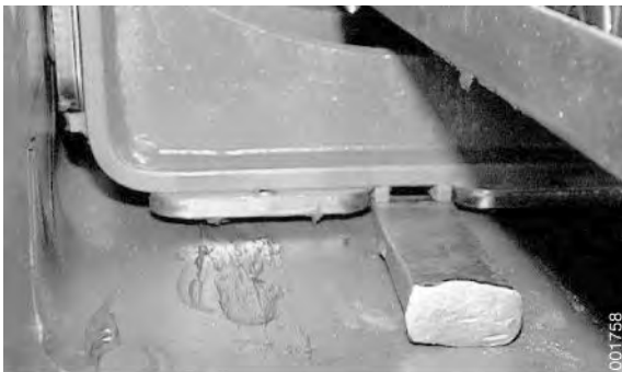
The diagram shows inner slide plates in the attachment's main beam.
