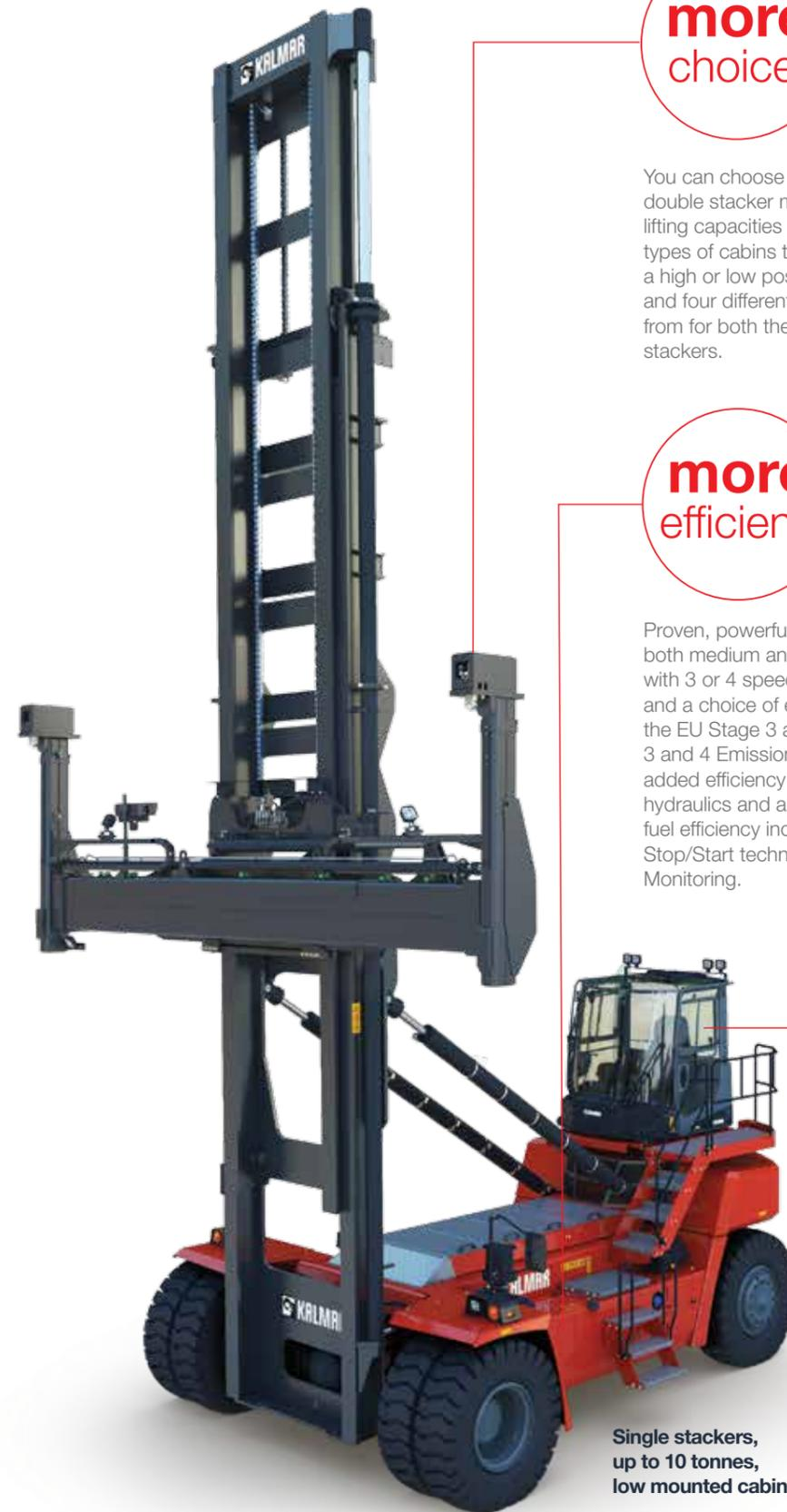
Single stackers, up to 10 tonnes, low mounted cabin.
