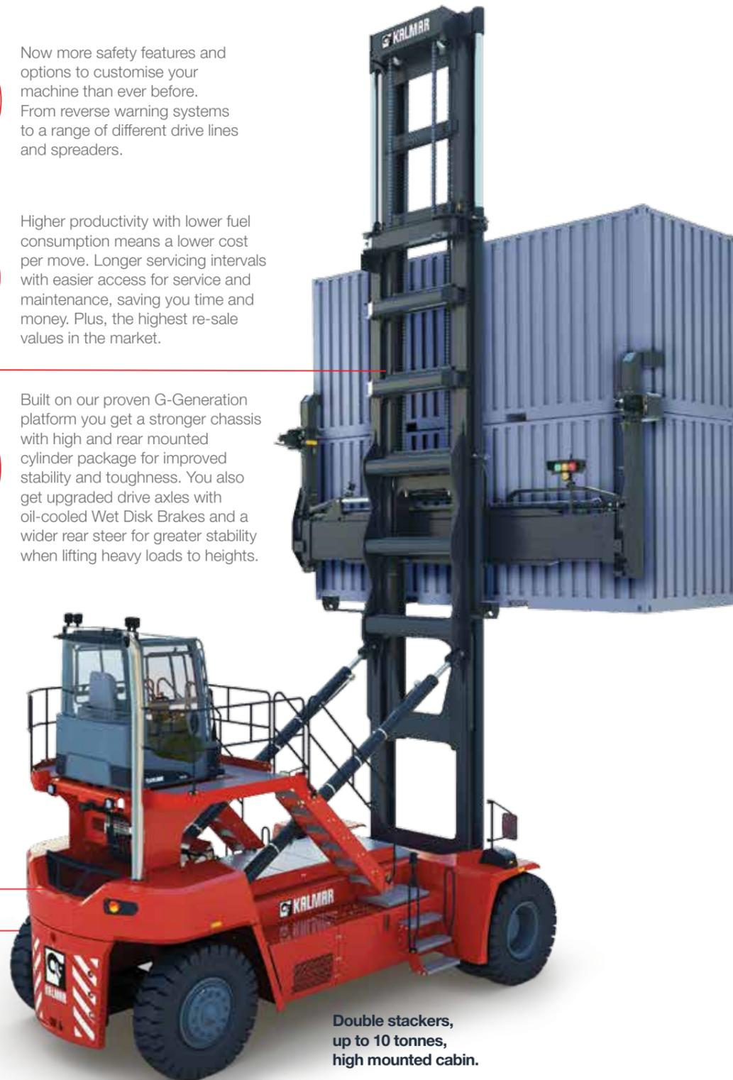
Double stackers, up to 10 tonnes, high mounted cabin.
