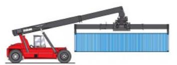
It's easy to lift containers lengthwise from a low, longitudinal position – through workshop doors, port shed gates and other tight openings.
