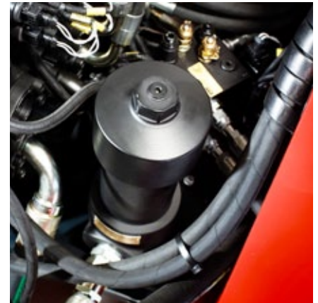
Improved placement of hydraulic filters.
